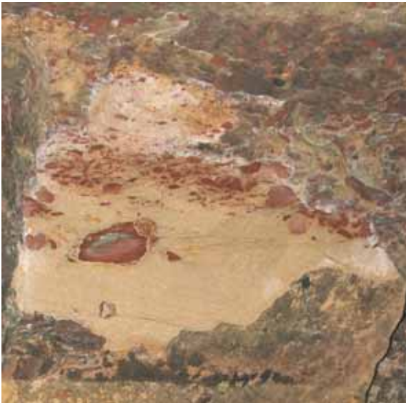
A small roof fall in the Brewhouse Yard caves exposed an abundance of red clay flakes within the sandstone; these caused the fall by their swelling with absorption of groundwater in the normal course of weathering.
